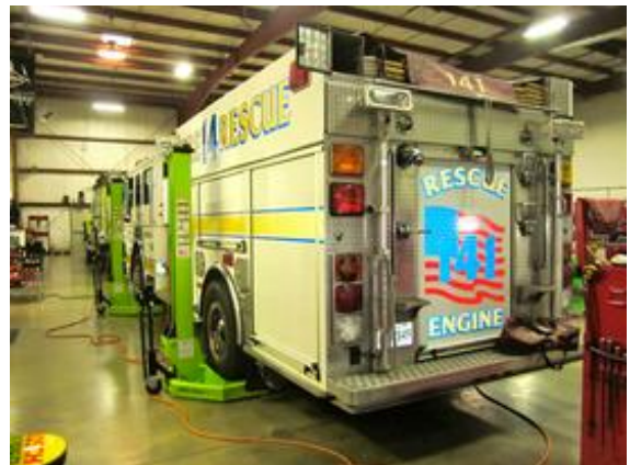
Engine 141 - a 1999 New Lexington pumper on an American La France chassis equipped with a Hale Q-Max 1500 gpm pump.
